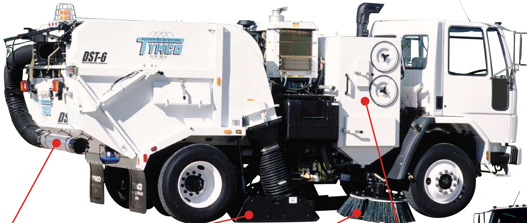
TYMCO's Broom Assist Pick-up Head (BAH®) with DUO SKIDS® gives you a full 87 inch sweeping path. With in-cab controls that allow broom-assisted sweeping only when needed.
